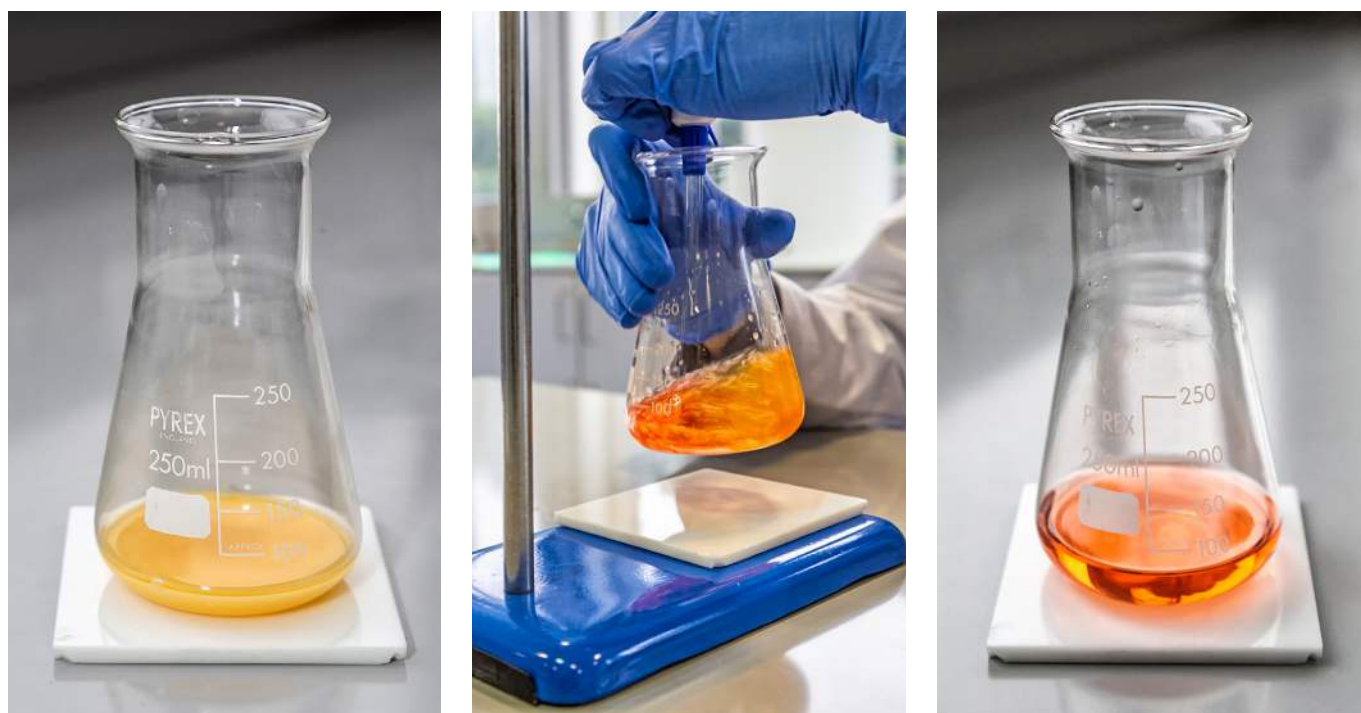
Figure 3 The sample solution (from left to right) at the beginning, the middle and just at the endpoint of the titration
